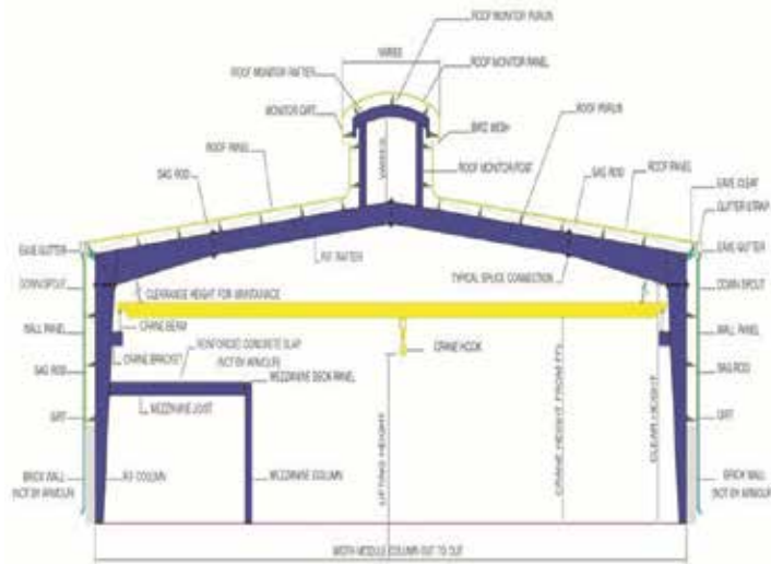
CROSS SECTION - RIGID FRAME CLEAR SPAN
